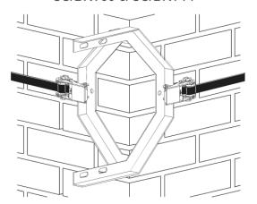
Fit a suitable aerial mast to the bracket using V bolts. It may be necessary to use a cranked mast if the chimney has a stepped top (avoid positioning the aerial over the top of an operating chimney as heat and gas may affect performance over time).
